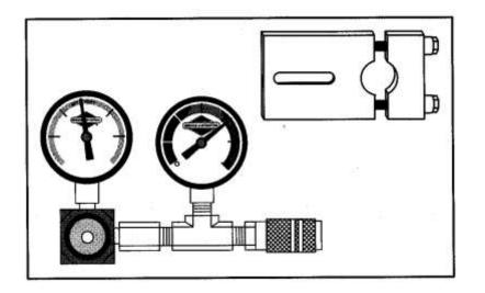
Basically you insert the device in place of your engines spark plug, fill the cylinder with compressed air and the leakdown tester measures any air leaks.
