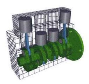
Also as we learned earlier pistons are manufactured slightly smaller in diameter than the bore of the particular engine and then rings are installed to maintain proper compression.
